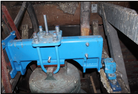
This photo shows the new headstock and bearings fitted to bell number four. It is hoped that, if we can fund a new frame for the bells, the two new headstocks can be reused in the new frame.
