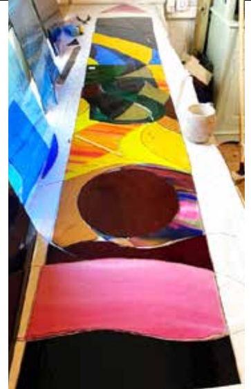
Figure 3 The glass is cut and placed on the cartoon for the right-hand light (Ch.3).
