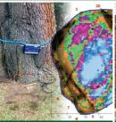
Advanced decay detection equipment to check internal integrity of a tree
