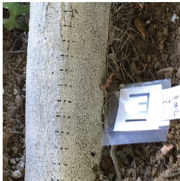
Figure 4. RSTZ and root prepared for sampling with painted surface and 2.5-cm reference lines on root.
