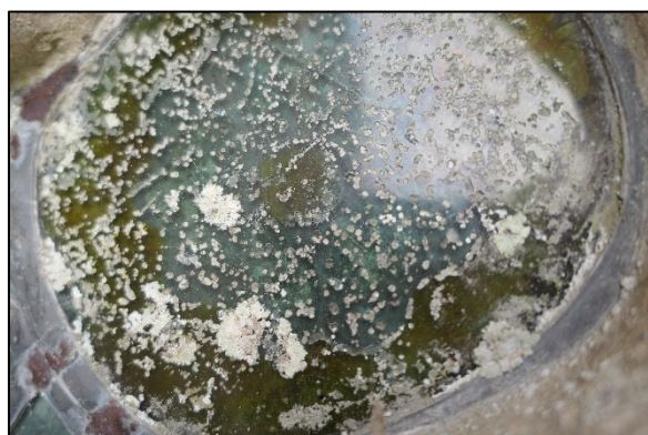
Fig.17 – Pitted exterior surface of lobe in 2b, dirt, corrosion products and lichen colonies.
