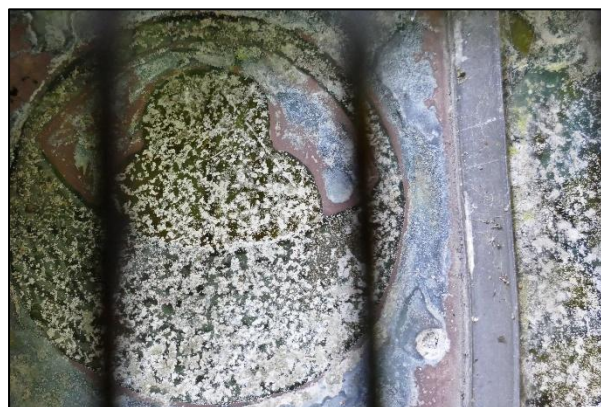
Fig.9 - Corroded back painting and pitted glass surface with white corrosion products, ext. of escutcheon, 2b.
