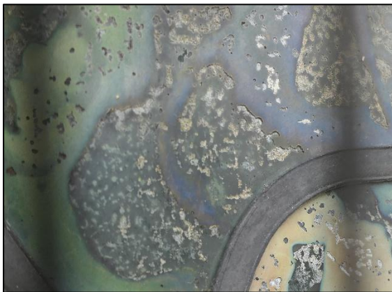
Fig.10 – Corrosion pits conjoining causing areas of surface loss, ext. of panel 1a.
