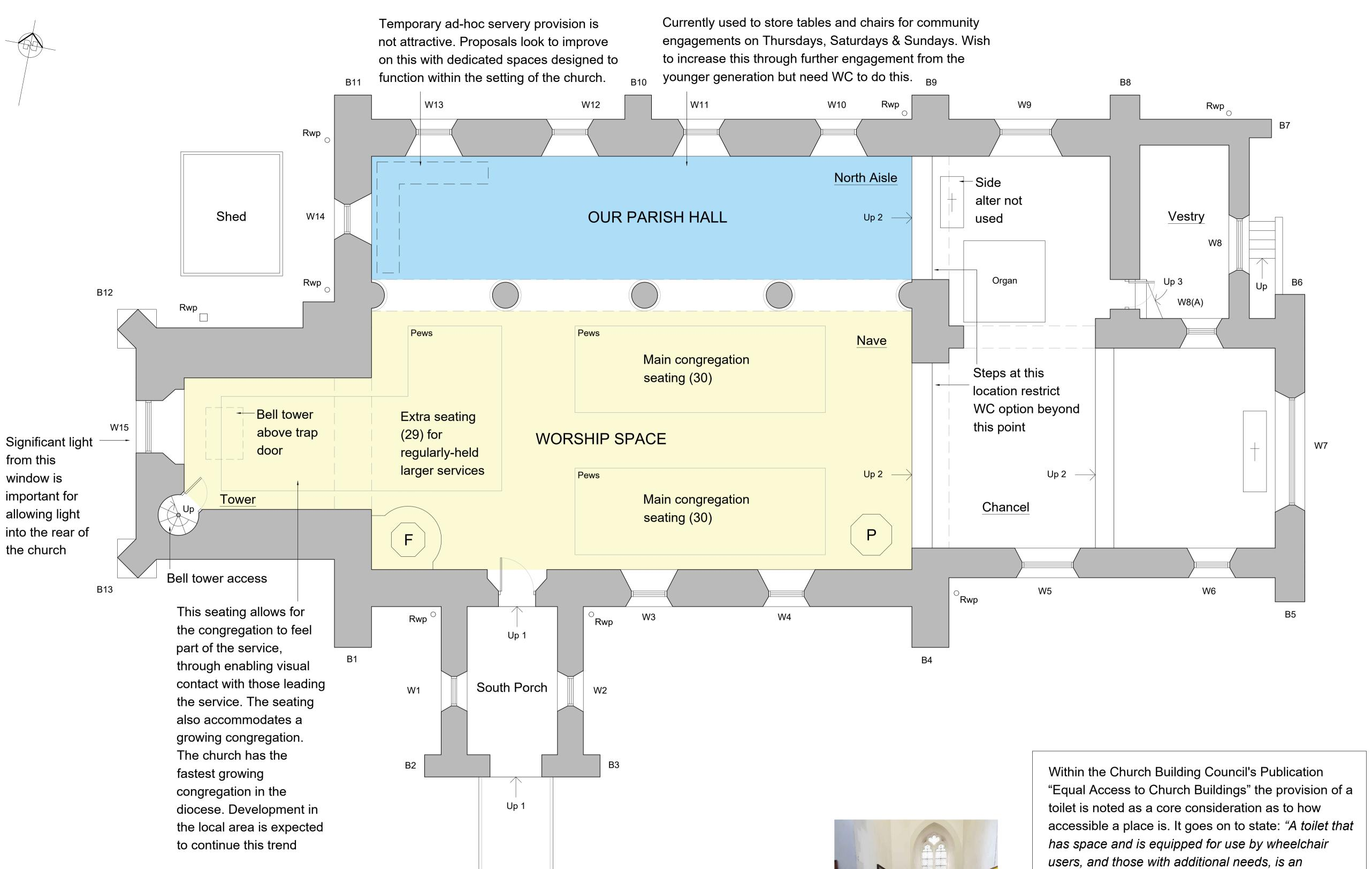
demonstrating how tower is used to accommodate
